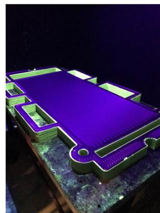
Crack detection of plates
